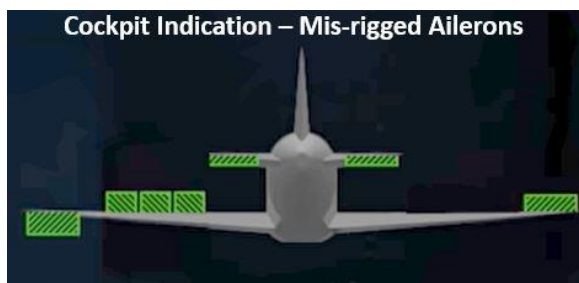
Figure 1 Cockpit Indications - Roll Control Movement
